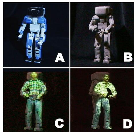
Fig. 8 (A) Miniature of the HONDA Humanoid Robot, (B) Painted with Retro-reflective Material, (C) Example of Projecting a Human onto it, (D) Another Example (adopted from [24]).
