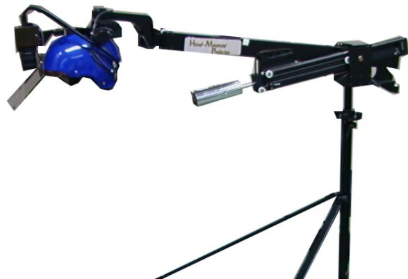
**Fig. 10 General View of Head-Mounted Projector (HMP) suspended by Counter-balanced Goniometer with 6-DOF. [27]**
