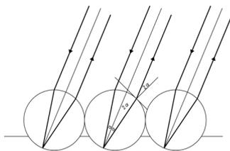
Fig. 15 Retro-reflective surface densely covered with microscopic beads with about 50 micrometer diameter. Ideally, the refractive index should be 2.
