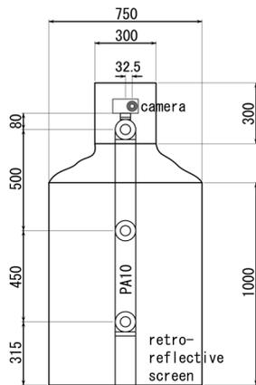
Fig.12 Configuration of Retro-reflective Screen Robot.
