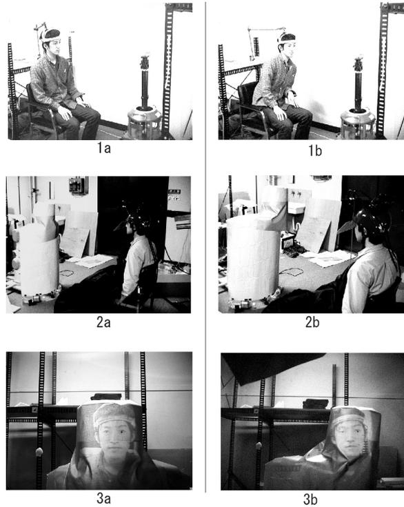
Fig. 13 Experimental Results: (1a, 1b) Human User A at Local Cockpit(A), (2a, 2b) Human User B and Telexistence Robot A' in Environment[B], and (3a, 3b) the image of the human user A on the robot A'. A black dot is where the camera is located.
